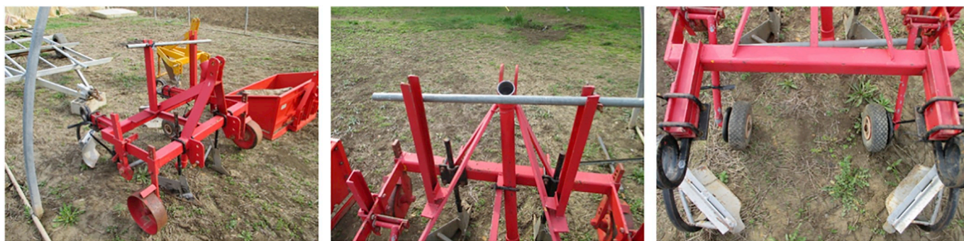
Fig. 6. Picture of an implement designed on farm and shared on the forum with a farmer's testimony: "This is my plastic mulch layer on a mini-cultivator base ... it lays 1m wide plastic film with drip irrigation under the mulch [...] I spent about two days on it, but thinking it out took much longer than that! I decided to build this plastic mulch layer because I couldn't find a second-hand one. As to price, it's all salvaged scrap [...] gas bottles, a piece of an electricity pole, weight lifting bars found on a waste tip, [...] all I had to pay for was welding rods, two wheelbarrow wheels and the paint."
